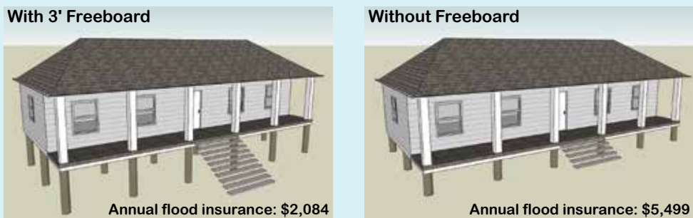
Figure 2-8. In this example, adding a small amount of height has very little effect on the look of a home, but results in a substantial flood insurance savings. 24 Image courtesy of Dan Gihring for StormSmart.org
