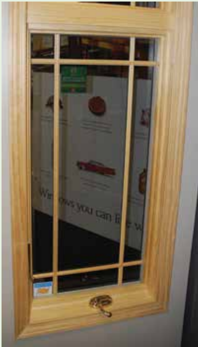
Figure 5-19. This attractive window can be fitted with energy-efficient glass, impact-resistant glass, or both. The impact-resistant glass consists of a laminate or film sandwiched between two glass panes. The frames are reinforced and the hinges have extra fasteners to withstand high-wind events. Wind-generated debris may crack the glass, but the laminate will hold the windowpane together in the frame and prevent breaching of the wind- and rain-resistant envelope. After the storm, the glass will need to be replaced. Image courtesy of Dennis Hwang
